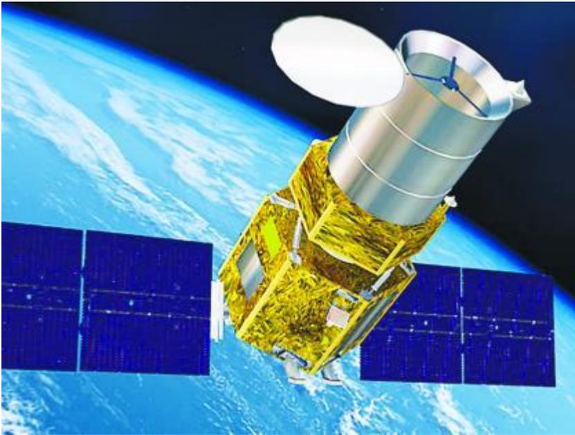
Built on Boeing's Phoenix platform, the HySpecIQ satellites will weigh 600 kilograms apiece and will be launched into a sun-synchronous polar orbit with an altitude of 500 kilometers. Credit: Boeing artist's concept
